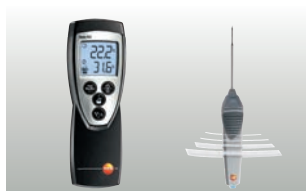
Wireless measurement with radio probes
