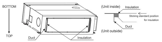
(\*) After unpacking, bottom side of the unit is located at the upper side.
